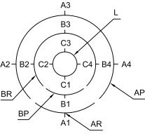
BR - Return Line For Cylinders In Clamped Position
